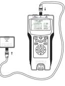
• Method.2: Connecting TEL Cable between MAIN with TERMINATOR for test. Connecting the TEL(6C° 4C° 2C)Cable between MAIN with TERMINATOR for test.
